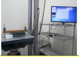
Mechanical Shock Test: +Z axis
